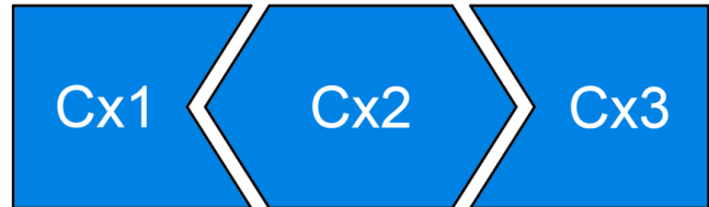
Figure 6.1 : Self Capacitance Swipe Switch Sample Electrodes.
